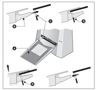
Figure 4: Attaching/Detaching the Feed Table
